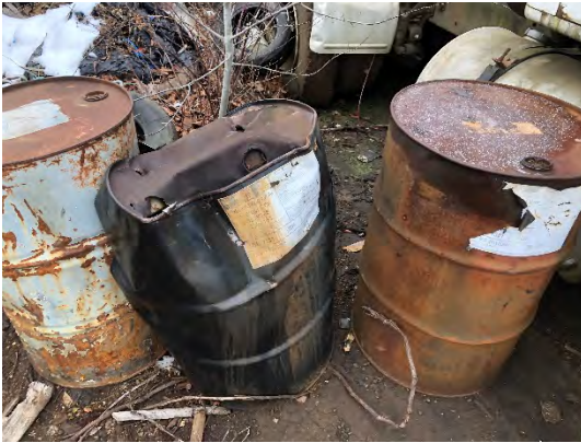
Photograph 47: Three 55-gallon drums with stained soils.
