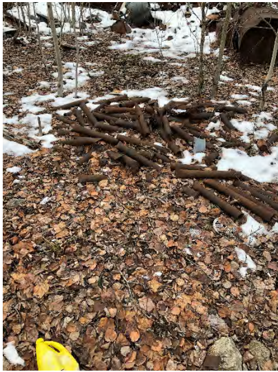
Photograph 97: TENORM pipe sections.
