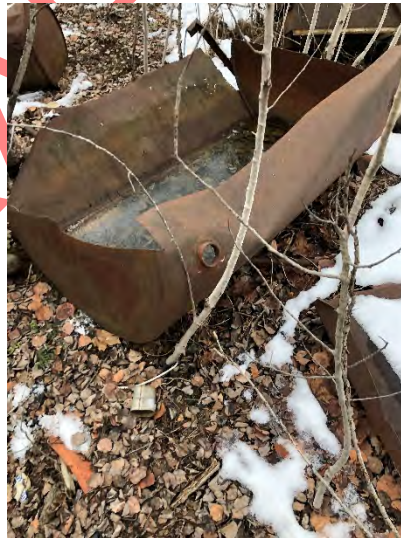
Photograph 100: Split old UST.
