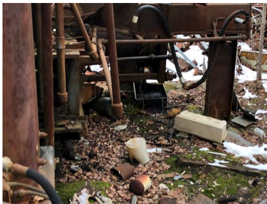
Photograph 67: Buckets catching fluids under scrap yard equipment.
